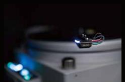
Traditional MM & MC cartridges rely on magnets and coils to generate the electrical signal. The optical cartridge uses a beam of light to detect cantilever movement, making the cartridge much lighter and more agile in tracking the record groove. With the coils, magnets, and magnetic field of a conventional cartridge removed—and its subsequent influence on cantilever movement and sound quality, the optical cartridge produces the most natural sound from vinyl LPs.
